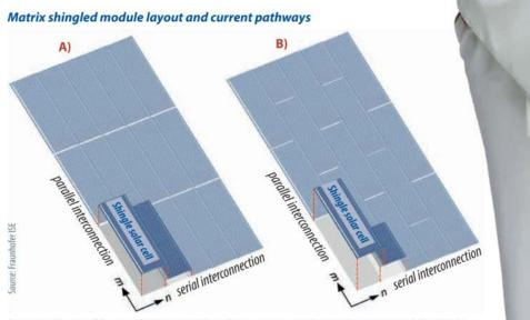
Schematic drawing of the two shingling approaches: A) string-type in which n serial-interconnected shingle solar cells form m parallel-interconnected strings, and B) in matrix-type in which each of the n serial-interconnected rows contain m parallel-interconnected solar cells by shifting cells by half their length perpendicular to the stringing direction. Half-cut shingle solar cells are also placed at the edges to complete a regular rectangle.
